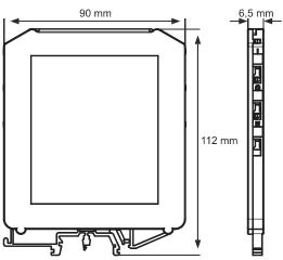
E-790 device control units are designed for rail mounting and should be used in an industrial environment.
