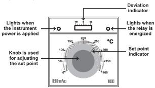
The Connection diagram are defined in 5. section. 220 V AC is applied on 1 and 2 terminals. Pls. contact us on order if you use 110 V AC. Relay connections are made terminals 3 (NO), 4(O) and 5(NC). When the power is applied to the instrument the green led on the upper left side of the panel becomes on. Set point adjustment with knob in the middle of the instrument. The red led on the upper right side of the panel is on when the process
