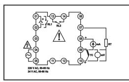
The labels on the sides of the controller identify the ordering code (Type), serial number and wiring connections. The controller options are also indicated on the wiring diagram.
