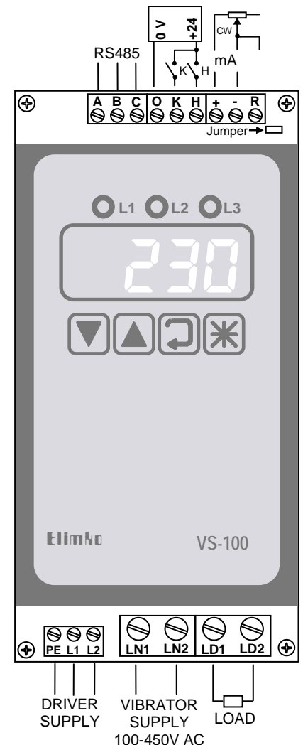
Figure 2.1. Front Panel View of E-VS-100 and Connection Terminals.
