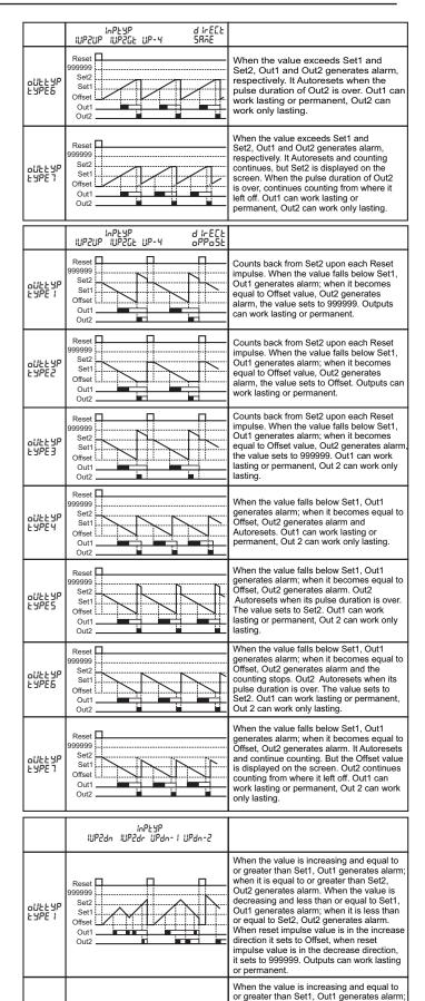
when it is equal to or greater than Set2, Out2 generates alarm. When the value is decreasing and less than or equal to Set1,
