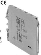
The input signal of E-790 series converters can be ordered as 0 - 1 A AC/DC or 0 - 5 A AC/DC and the output signal can be ordered as 0 / 4 - 20 mA or 0 - 10 V.
