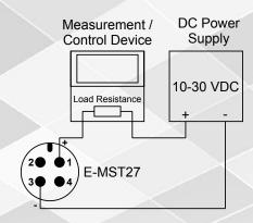
(\*\*) Pins 2 and 4 of the M12 socket are used for the configuration of the transmitter and should not have any external connections. Connecting to these pins can potentially damage the device.
